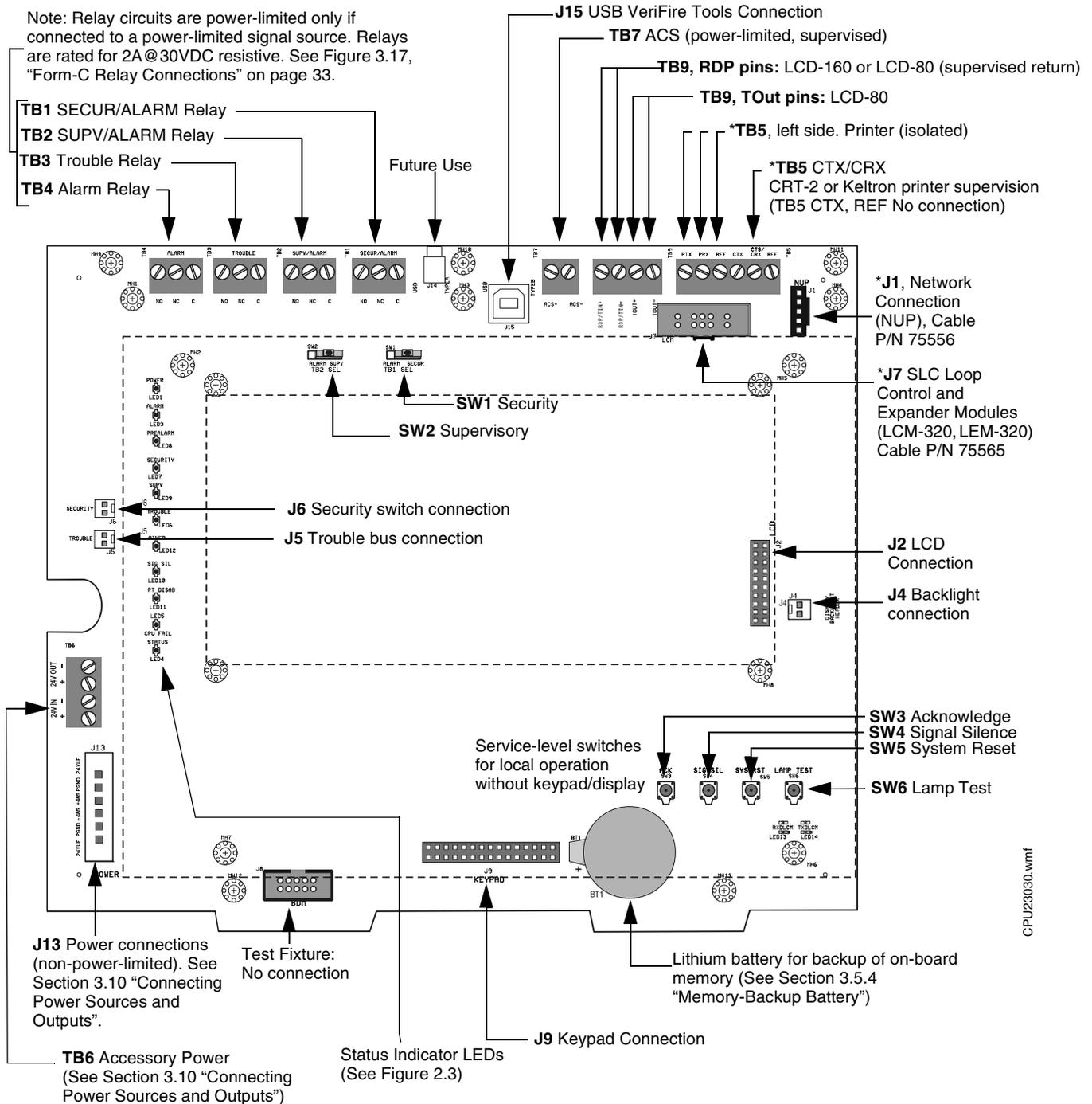
Figure 2.1 CPU Connections
