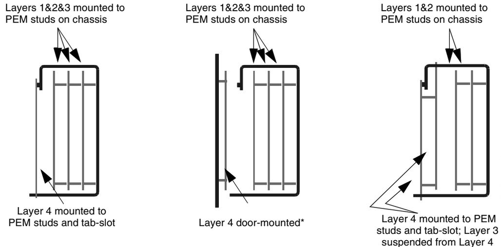
\*Note: If CHS-4N is used, door-mounting is only for use with ACM-24AT and ACM-48A series annunciators.
