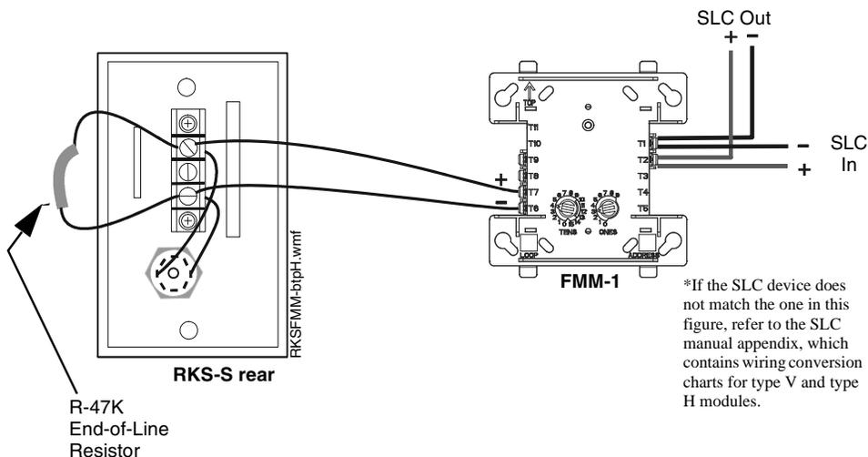
Figure 4.8 Connecting the FMM-1 Module to the RKS-S
