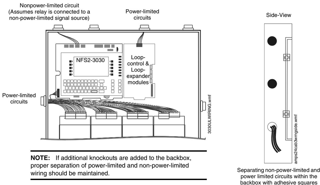
Figure 3.19 Typical Wiring in a Four-Row Backbox
