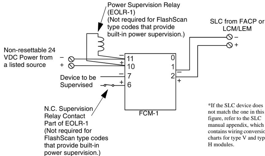
**Figure 4.1 Enabling External Power Supervision Using Relays**
