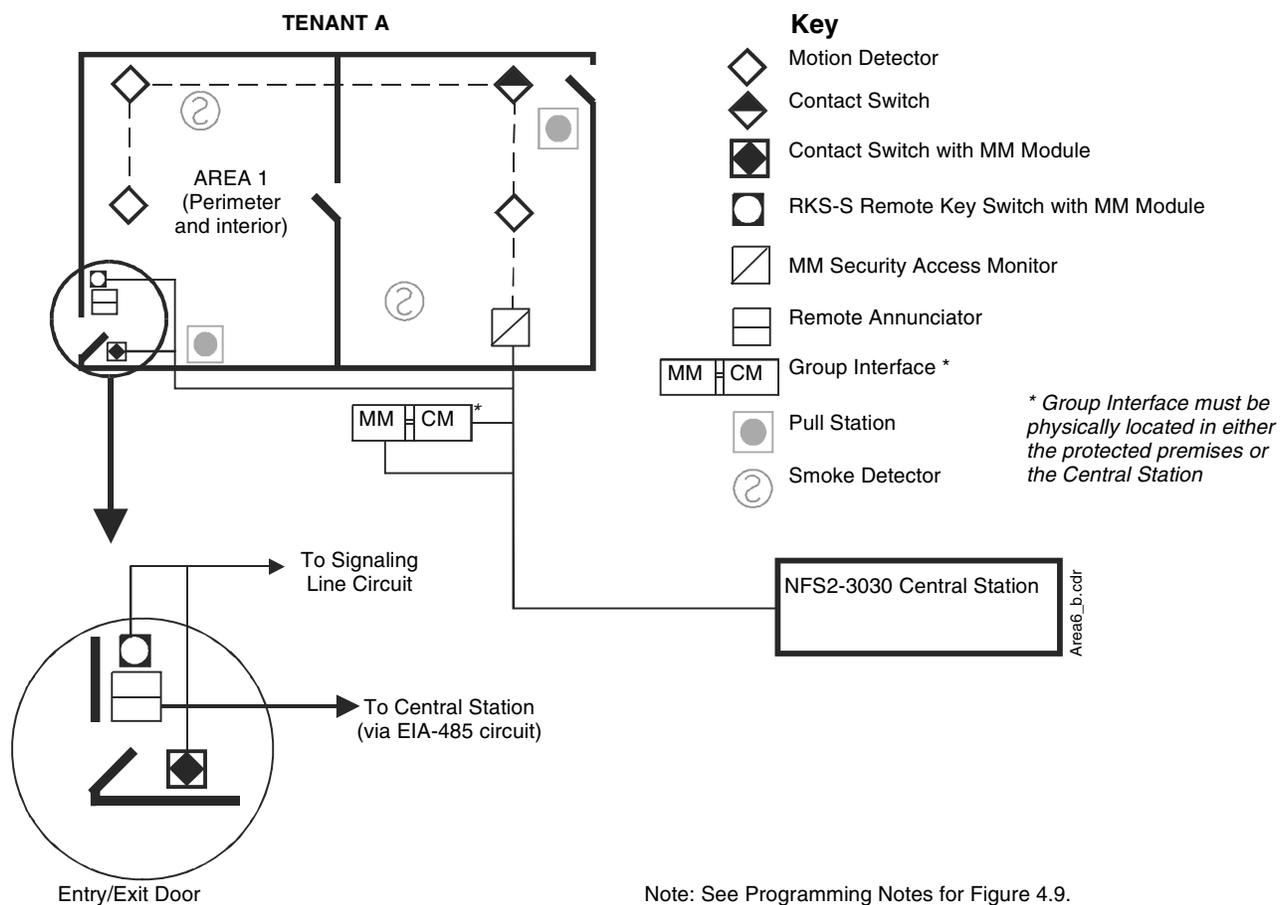
**Figure 4.9 Single Tenant Security System with Entry/Exit Delay**
