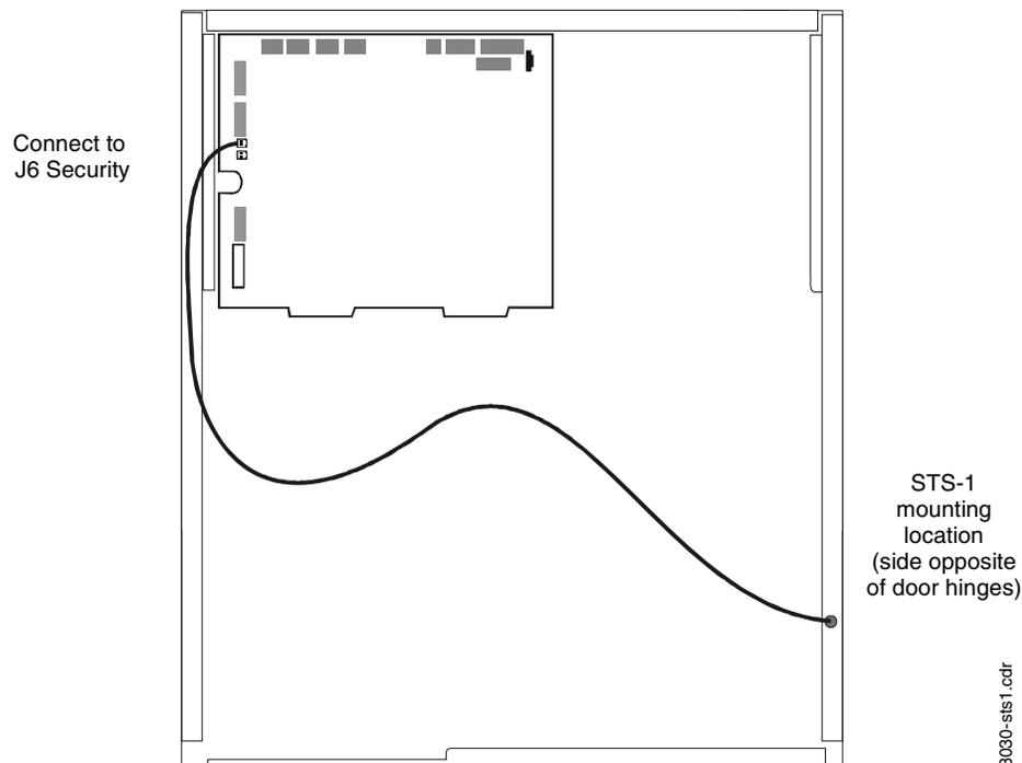
**Figure 4.5 Installing the STS-1 Security Tamper Switch**
