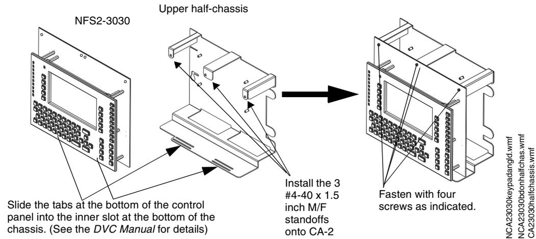
**Figure 3.7 Mounting the NFS2-3030 onto the CA-2 Half-chassis**
