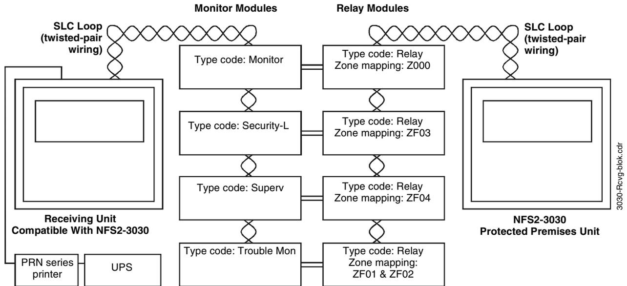
Note: Remote printers require 120 VAC, 50/60Hz primary power. A secondary power source (battery backup) is not provided; the use of a separate Uninterruptable Power Supply (UPS) 50 watt minimum, UL-listed for Fire Protective Signaling is recommended. A UPS is required for NFPA 72 Proprietary Protected Premises Receiving Unit Applications.
