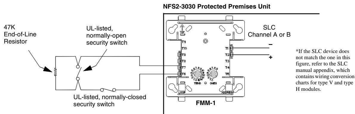
Figure 4.6 Wiring Diagram for Proprietary Security Alarm Applications
