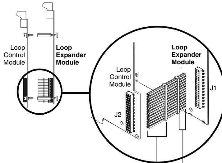
The long-pin end plugs directly into the back of the Loop Control Module board.
