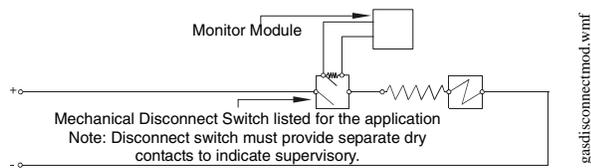
**Figure 4.12 Typical Connection of a Mechanical Disconnect Switch**
