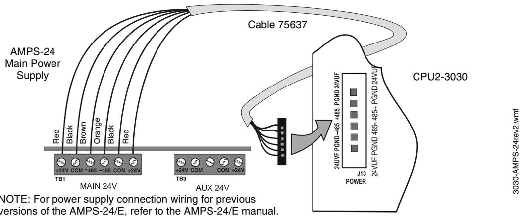
**Figure 3.18 DC Power Connections: Main Power Supply**
