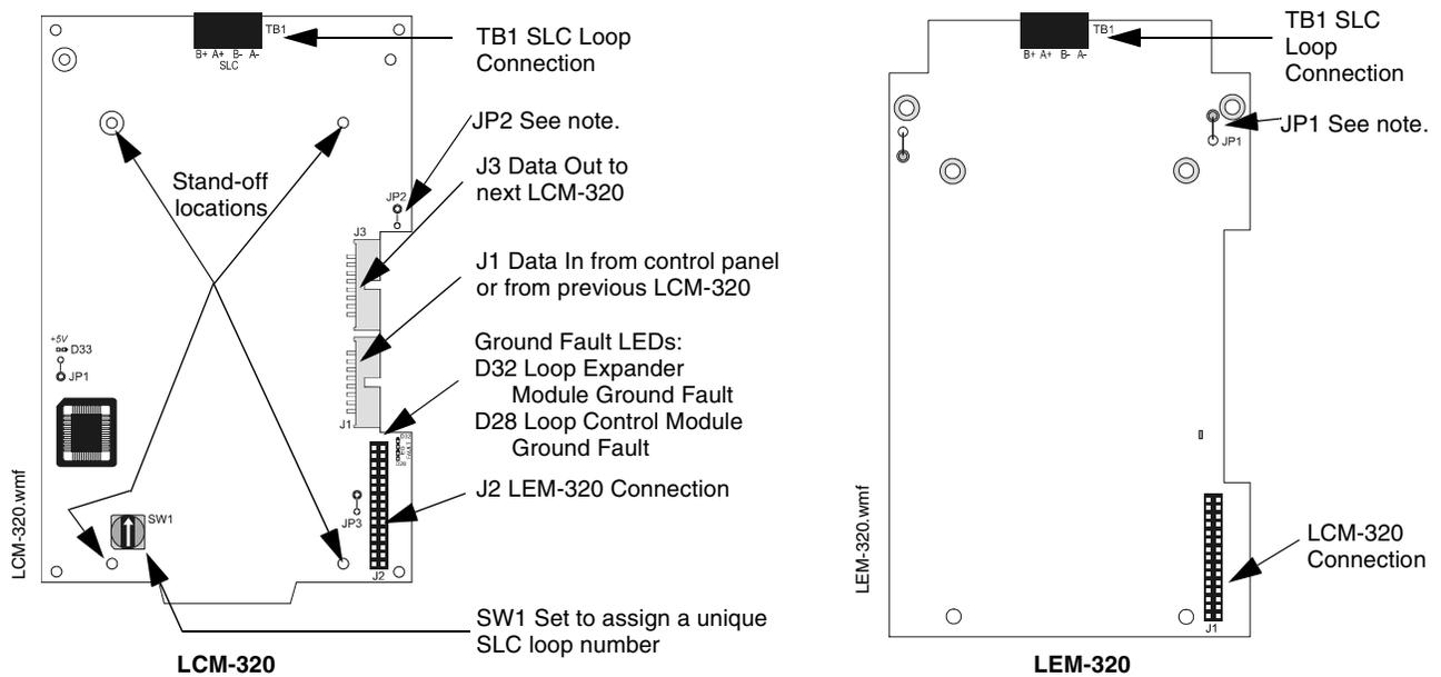
**Note:** Do not cut any jumpers on the LCM-320 or LEM-320.
